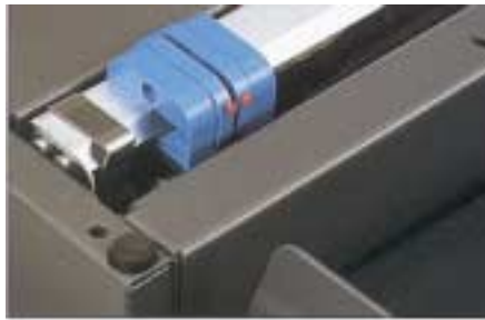
Two high-performance reading heads to verify mark accuracy.
